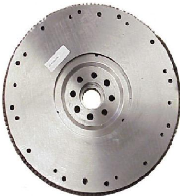
FORD FWNE7HZ6375A Style: FLAT Application: 6.6L / 7.8L Clutch: 14+ . 8 spring disc Bearing: #206 / 305 7.125+bore, 8 mounting holes 17+ring gear with 138 teeth List Price $579.94
