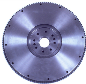
CATERPILLAR FWN9Y9311 Style: FLAT Application: 3208 Clutch: 14" – 8 spring disc Bearing: #206 / 305 7.125" bore, 8 mounting holes, 2 dowel holes Thickness: 1.525" 17" ring gear with 134 teeth List Price $479.46
