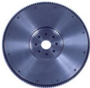
NAVISTAR FWN1810855C93 Style: FLAT Application: DT466 (A, B & C) Clutch: 14" – 8 spring disc Bearing: #205 7.125" bore, 8 mounting holes Thickness: 1.675" 17" ring gear with 138 teeth List Price $281.36
