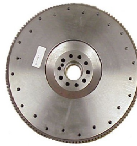
NAVISTAR FWN1818214C91 Style: FLAT Application: 7.3L 444E Clutch: 13" or 14" - 8 spring disc Bearing: #206 / 305 7.125" bore, 10 mounting holes, 1 dowel hole Thickness: 1.835" 17" ring gear with 137 teeth List Price $373.23
