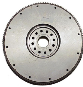
NAVISTAR FWN1821915C91 Style: FLAT Application: DT466E Clutch: 14" – 8 spring disc Bearing: #206 / 305 7.125" bore, 12 mounting holes Thickness: 1.500" 17" ring gear with 138 teeth List Price $307.20
