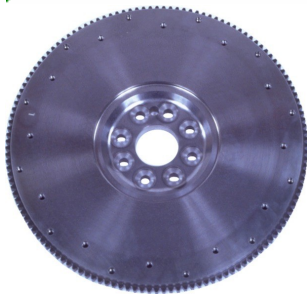
CATERPILLAR FWN1265875 Style: FLAT Application: 3116 / 3126 Clutch: 13" or 14" Bearing: #206 / 305 8 mounting holes, 1 dowel hole Thickness: 1.525" 17" ring gear with 134 teeth List Price $339.90
