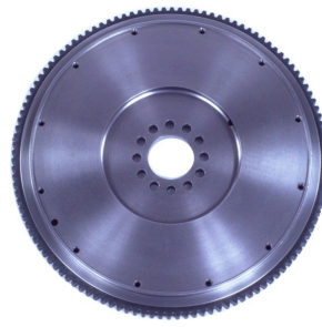
CATERPILLAR FWN4P4797 Style: FLAT Application: 3406 / 3406E Clutch: 15" - 7 or 10 spring disc Bearing: #306 10" bore, 12 mounting holes, 1 dowel hole Thickness: 1.830" 20" ring gear with 113 teeth List Price $617.27
