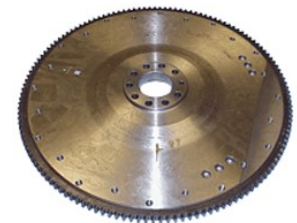
NAVISTAR FWN1809144C91 Style: FLAT Application: 6.9L / 7.3L Clutch: 13" or 14" - 8 spring disc Bearing: #205 7.125" bore, 9 mounting holes, 1 dowel hole 17" ring gear with 137 teeth List Price $387.48
