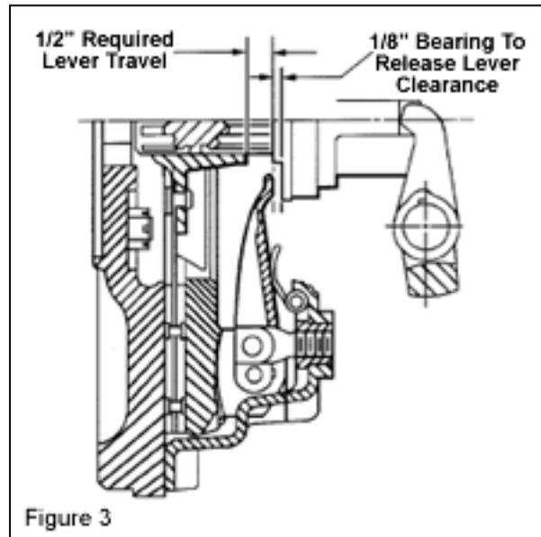
5. If excessive free play is present in the clutch pedal linkage due to worn parts, the worn parts must be replaced. Excessive wear of the release linkage may give a false impression of the actual amount of release bearing clearance.
